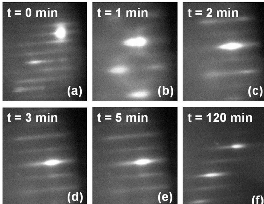
Fig. 1. (a) GaSb  $(1 \times 3)$  reconstruction before the growth of ZnTe. (b) Spotty RHEED pattern within the first minute of ZnTe growth on GaSb. (c)–(f) ZnTe  $(1 \times 2)$  reconstruction after 1 min growth and longer.
