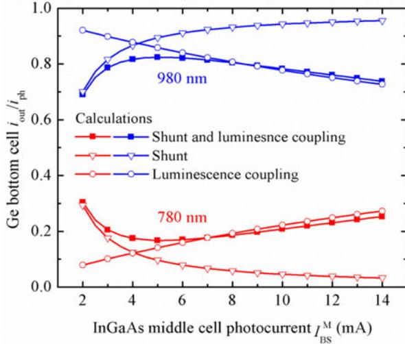
Fig. 7. Calculated  $i_{\text{out}}/i_{\text{ph}}$  of Ge bottom cell at 980 and 780 nm with shunt and luminescence coupling (squares), with only shunt (open triangles) and only luminescence coupling (open dots) when the InGaAs photocurrent  $I_{\text{BS}}^M$  is increased.
