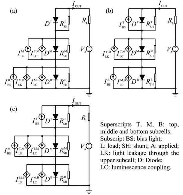
Fig. 2. DC equivalent circuits of a triple-junction solar cell at the voltage and light bias conditions of EQE measurements for (a) the top subcell, (b) middle subcell, and (c) bottom subcell.
