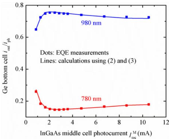
Fig. 6.  $i_{\text{out}}/i_{\text{ph}}$  extracted from Fig. 1 (dots) and calculated using (2) and (3) (lines).
