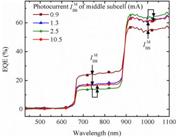
Fig. 1. EQE spectra of the Ge bottom cell of a triple-junction solar cell at the reverse-bias voltage of  $-0.45$  V and under different bias light intensities and photocurrents  $I_{BS}^M$  generated in the InGaAs middle cell.
