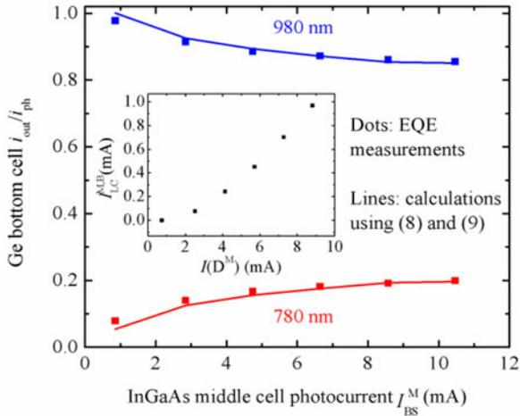
Fig. 4. Fitting of  $i_{\text{out}}/i_{\text{ph}}$  of the Ge bottom cell obtained from EQE measurement (dots) with those from calculations (lines) using (8) and (9) at the optimal bias voltage of 0.2 V (forward bias) when the InGaAs photocurrent  $I_{\text{BS}}^M$  is increased. The inset shows the luminescence coupling current  $I_{\text{LC}}^M$  from the InGaAs middle cell to the Ge bottom cell versus the recombination current  $I(D^M)$  of the InGaAs middle cell.
