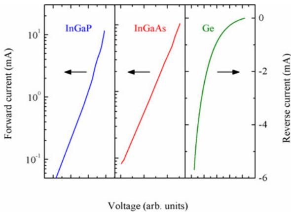
Fig. 5. Measured forward dark  $I$ - $V$  curves of the InGaP and InGaAs subcells and reverse dark  $I$ - $V$  curve of the Ge subcell.
