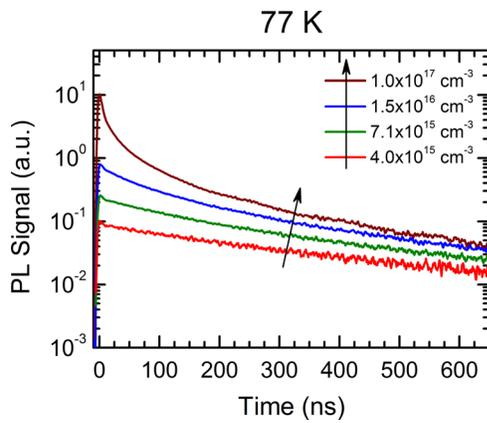
FIG. 1. (Color online) Time-resolved photoluminescence measurements on an InAs/InAs<sub>0.72</sub>Sb<sub>0.28</sub> T2SL at 77 K for initial excess carrier densities ranging from  $4.0 \times 10^{15}$  to  $1.0 \times 10^{17} \text{ cm}^{-3}$ .
