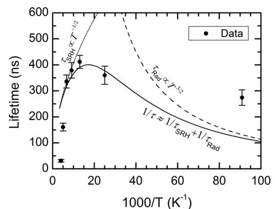
FIG. 3. Carrier lifetimes extracted from the fits in Fig. 2 of the PL decay are shown as points as a function of  $1000/T$ . Also plotted is the temperature dependence of the SRH lifetime ( $\tau_{\text{SRH}} \propto T^{-1/2}$ , dotted line), radiative lifetime ( $\tau_{\text{Rad}} \propto T^{3/2}$ , dashed line), and a combination of both SRH and radiative lifetimes (solid line).
